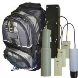
Gambar 1c. Backpack Detektor Gamma - Neutron
