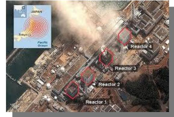
2011 - Fukushima reactor flooded by tsunami and damaged the plant's 5 active reactors. Loss of backup electrical power led to overheating, meltdowns, and explosion
