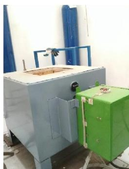
Gambar 2.2 Prototipe TOLACORE apparatus corrosion test
