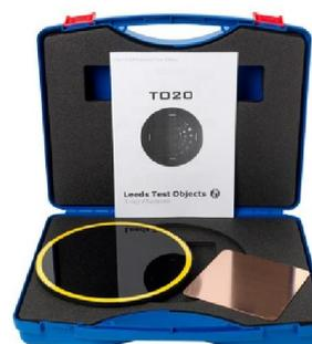
Gambar 2. *Leeds Test Phantom Low Contrast TO 20*
