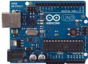
Gambar 4. *Board* Arduino Uno<sup>[1]</sup>.
