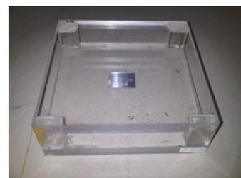
Gambar 3. *Leeds Test Object (High Contrast)* dan *Phantom*
